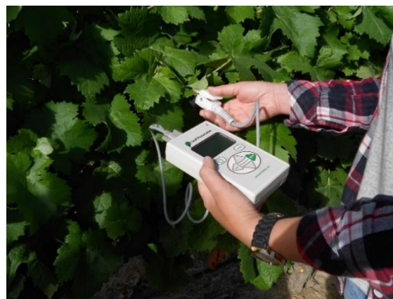
Figure 2. Stomatal conductance measurement using a leaf porometer. Source: Salgado-Pirata (2018).
